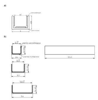
Fig. 12. Connectors BP11 Ł H1 (a) and BP11 Ł H2, BP11 Ł H3, BP11 Ł H5 (b)
