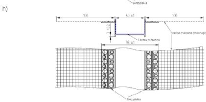
Fig. 6. Beads BP11 H1S (a), BP11 H2S (b), BP11 H3S (c), BP11 H3 NS (d), BP11 H5S (e), BP11 H2 RS (f), BP11 H3 RS (g), BP11 H5 RS (h)
